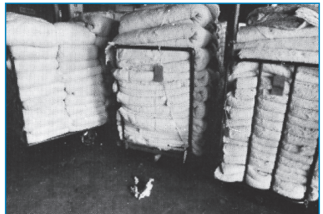
CLASS III, DIVISION 2 STORAGE AREA.
