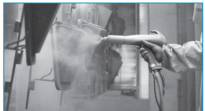
PAINT BUBBLES, DRIPS AND OTHER SURFACE IRREGULARITIES ARE VIRTUALLY ELIMINATED SINCE POWDER, RATHER THAN A LIQUID PAINT, IS APPLIED ELECTROSTATICALLY.
